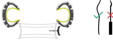
1. Make sure your spoke nuts are well protected with rim tape. If not, replace with new one or wrap it with duct tape.
