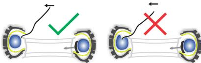
14. Mount second enduro tyre bead plus one Traxy Tyre Support bead together onto the rim. Start mounting at the Traxy Rim-lock and complete mounting at the Traxy Rim-lock. Make sure that Traxy Rim-lock stays in the middle of the Traxy Tyre Support.
