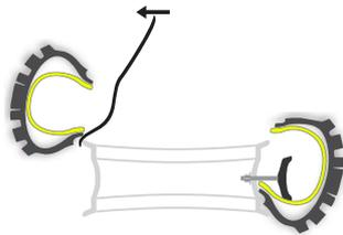
6. Mount one enduro tyre bead plus one Traxy Tyre Support bead onto the rim. Start mounting at the Traxy Rim-lock and complete mounting at the Traxy Rim-lock. Make sure both beads get under the Traxy Rim-lock.
