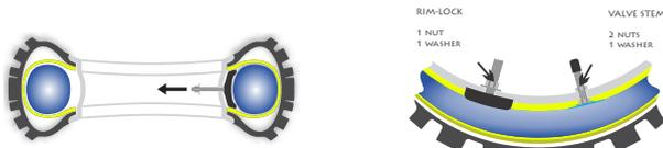
15. Inflate the tube to 1.5 .. 2 bar to get the tyre seated onto the rim bead. Check air tightness of the valve by putting saliva over valve hole.
