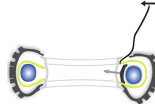
4. Remove one Traxy Tyre Support bead off the rim. Start next to the Traxy Rim-lock.
